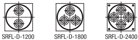
Detail arrangement of filter elements
