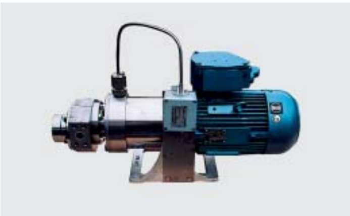
Gear pump with magnetic coupling ( hermetically tight ), explosion-proof motor, in cast steel, with temperature sensor (petrochemistry)
