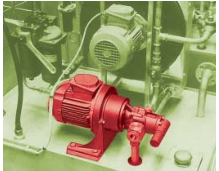
Gear pump SF in oil-supply installation
