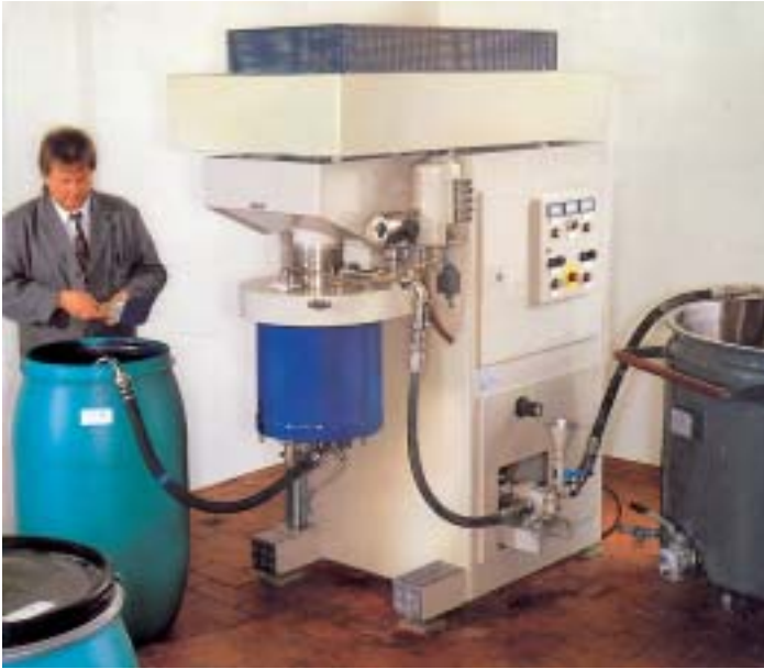
Gear pump in an agitating mill (Perl Mill)
