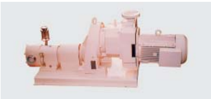
Rotary-lobe-pump unit with frictional-wheel control gear motor and axial face seal with unpressurised quench feed system for water-soluble paints and lacquers
