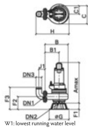
Dimensions - guide rail fitting type in mm:
