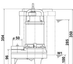
Dimensions - guide rail fitting type in mm:
