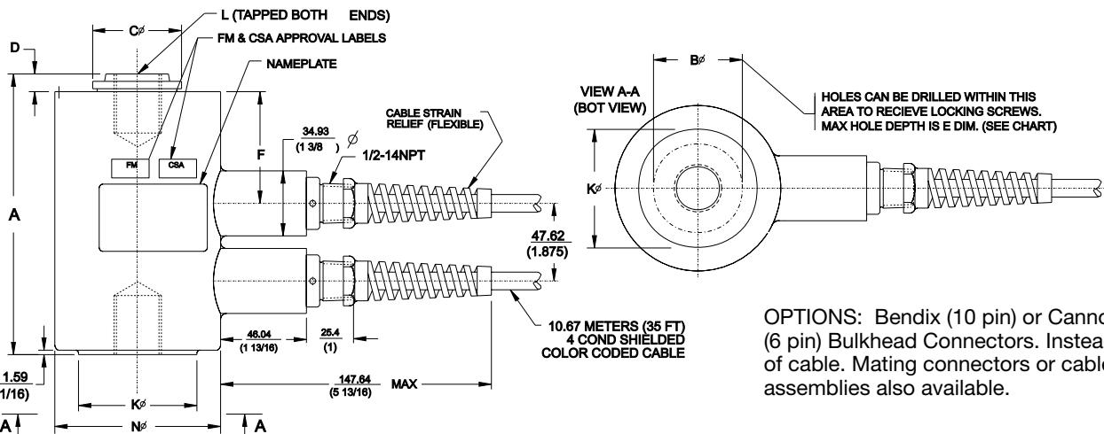
OPTIONS: Bendix (10 pin) or Cannon (6 pin) Bulkhead Connectors. Instead of cable. Mating connectors or cable assemblies also available.
