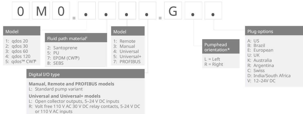
\* The pumphead side location is required when ordering. The left/right perspective assumes the user is looking at the front of the pump. The pump in the dimensions diagram is considered a pumphead located to the left.
