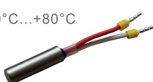
Sensors TF101U2 are encapsulated in a stainless-steel-shell V4A. They are suitable for measuring temperatures in fluids, at surfaces or for inside or outside applications. The protection class is IP 66. The version with PVC-insulated cable (3 x 0,25 mm<sup>2</sup> in one cable) can be easily wired. The maximum ambient temperature is 105 °C.
