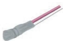
Platinum resistance temperature sensor on ceramic substrate protected by a heat-shrinkable sleeve and with PTFE isolated stranded wire. The TF101K version can be installed in motor or transformer windings. When build-in into windings do not pressure the sensor element. Precautions should be taken to protect sensor and extension leads against push and pull forces. Thermal response time  $T_{0,9}$  in the air 100 s, in water 19 s.
