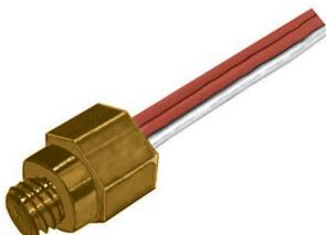
Platinum resistance temperature sensor on ceramic substrate built into a M6 brass threaded bush, especially suitable for being screwed into metal, e.g. for monitoring temperature of heat sinks or heating plates.
